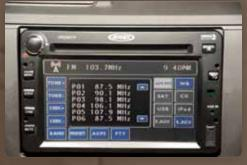
**Touch Screen Panel** Upgrade your RV Radio with a 6.5" LCD touch screen that functions both as the RV Radio controls and the color rearview monitor.
