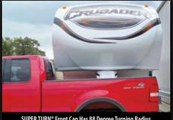
SUPER TURN® Front Cap Has 88 Degree Turning Radius
