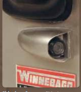
**Sideview Cameras** Sideview cameras activate with the turn signals and provide an added sense of comfort when maneuvering.
