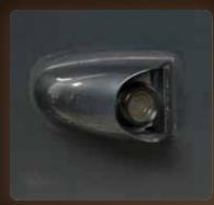
Available sideview color cameras activate with the turn signals and display on the dash-mounted LCD monitor to assist with maneuverability and visibility.
