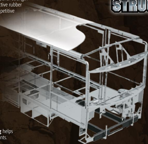
Specially engineered **interlocking joints** connect the floor, sidewalls and roof into a cohesive unit.
