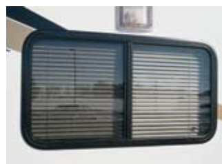
Automotive D-Seal around windows, no butyl tape
