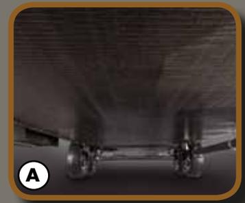
**A** Heated and Enclosed Underbelly (N/A Lite Models)
