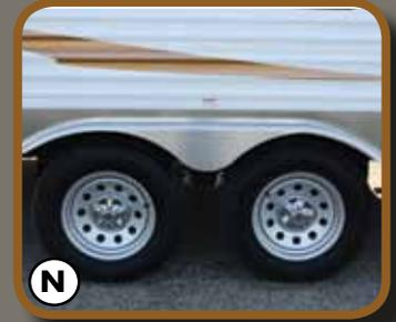
**N** SuperLube™ Axles with Radial Tires, polished aluminum fender skirts and E-Coat Wheels.
