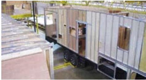
ALUMINUM STUDDED SIDEWALLS AND ROOF TRUSSES ON 16" CENTERS OR LESS
