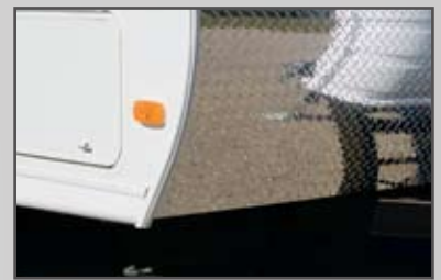
Diamond plate protected front wall adds protection against road elements and adds stylish flair.
