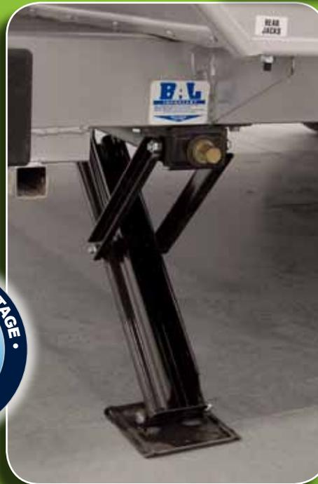
Rear stability jacks quickly and easily crank down to minimize movement in your MPG and speed up setting camp so you can get on with your vacation.
