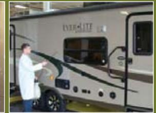
Seal Tech Leak Test
