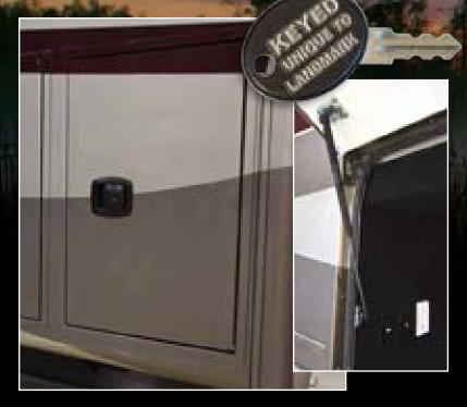
Enjoy the sleek, modern looks and functionality of LANDMARK's new optional bus style slam doors equipped with heavy duty struts for easy operation and they prevent unexpected closings due to wind. Oversized pull latches open easily. The tight automotive rubber seal protects your belongings from moisture and LANDMARK's compartments are keyed for security using keys and locks unique to LANDMARK.
