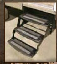
RADIUS ENTRY STEPS: These steps provide a safe entry into the North Country.The radius front edge eliminates the sharp corners and gives you more step for added safety.
