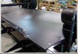
HEATED AND ENCLOSED UNDERBELLY This one-piece corrugated plastic underbelly is fitted and attached to the
