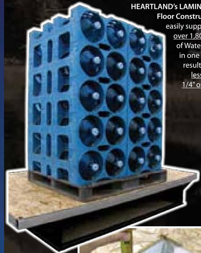
HEARTLAND'S LAMINATED Floor Construction easily supported over 1,800 lbs. of Water Jugs in one spot - resulting in less than 1/4" of flex!!
