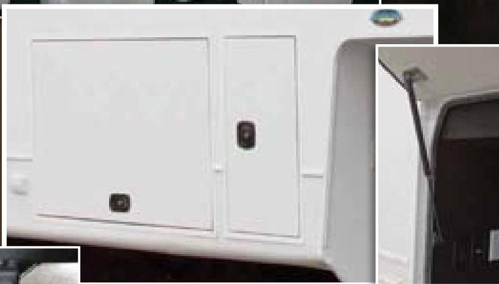
Enjoy the sleek, modern looks and functionality of BIGHORN's new optional bus style slam doors equipped with heavy duty struts for easy operation and they prevent unexpected closings due to wind. Oversized pull latches open easily. The tight automotive rubber seal protects your belongings from moisture and BIGHORN's compartments are keyed for security using keys and locks unique to BIGHORN.
