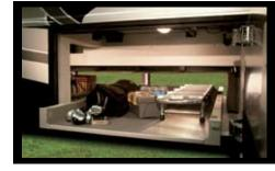
The Pass Through Storage Compartments allow you to grab your gear from either side of the coach. Optional slide-out trays provide easy access to items in the back of the compartment. These compartments are insulated and vacu-bonded to ensure your stored items are kept safe.
