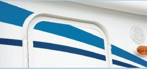
Radius entry door with drip cap
