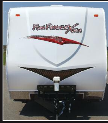
Front fiberglass cap with graphics, removable front storage tray and diamond plate rockguard.
