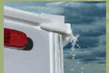
Another KZ standard – newly designed drip rails and spouts keep the water flowing away from the sidewalls.
