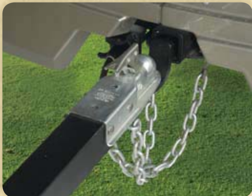
Hitch The 5,000-lb. hitch 5 with 7-pin wiring is perfect for your tow vehicle.
