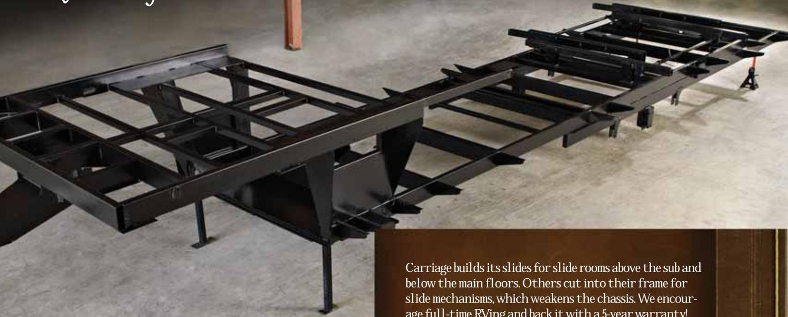
Carriage builds its slides for slide rooms above the sub and below the main floors. Others cut into their frame for slide mechanisms, which weakens the chassis. We encourage full-time RVing and back it with a 5-year warranty!
