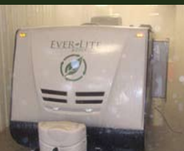
Rain Booth Testing 1/2" per minute
