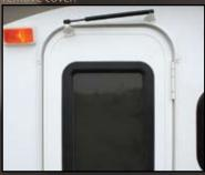
Radius exterior door with gas strut provides strength and durability compared to a square door with a plastic latch.
