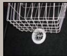
Ducted heat in the forward Pass Through compartment
