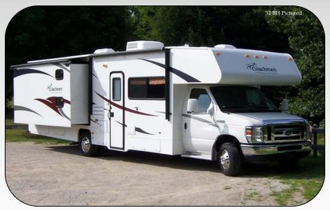
The Freelander provides easy access to the cab area with aluminum running boards. Azdel Superlite  $^{\text{TM}}$  sidewall material both, lightens the load & provides a smooth, durable fiberglass finish. Our standard slide-out awnings will keep rain and debris off the slides. At the end of the day, rest comfortably under the optional 12V power adjustable awning by A&E.
