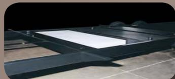
With Space Maker™ storage space is expanded by removing the freshwater tank from the interior of the unit. The Space Maker's location also lowers the center of gravity, improving towability. The heated compartment gives you added protection when cold climate camping.
