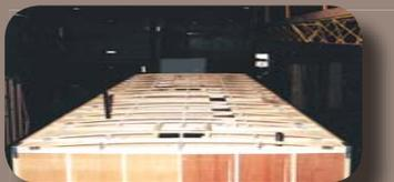
Springdale utilizes crowned, residential style, 41/2" truss rafters, shown here with air conditioning channels to accommodate our ducted roof/air option.
