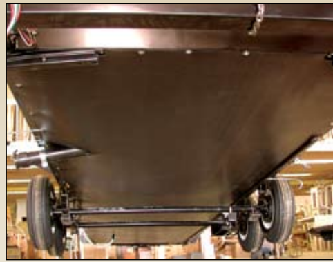
Sydney's heated underbelly encloses tanks and valves, helping to extend the camping season.
