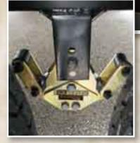
Trail-Air's EQUA-FLEX rubber-cushioned equalizer suspension system with shocks is standard on every BIGHORN and provides an incredibly smooth ride.
