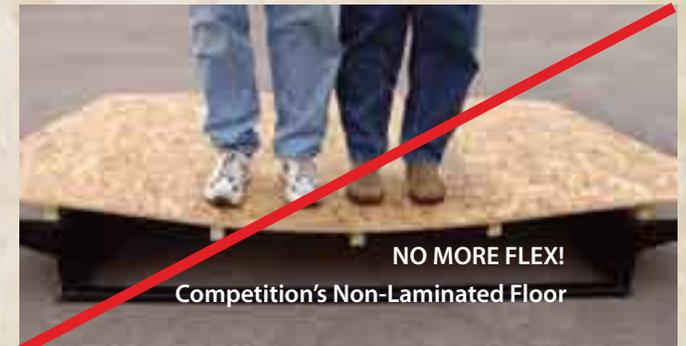
**Traditional RV Floor Construction** often flexes in the middle of the coach - because that's where the holding tanks are located and there is no steel frame support under the lumber.
