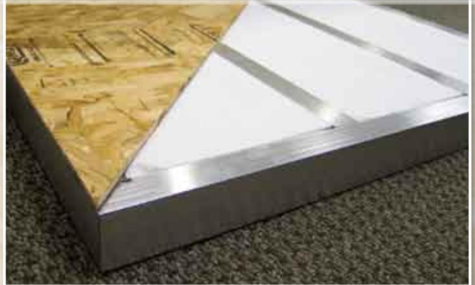
BIGHORN's LAMINATED Floor System is one of the **STRONGEST FLOORS** in the industry! Featuring sturdy 2.5" Aluminum Framing; thick Block Foam Insulation; One-Piece Seamless Decking and a Thermo-Board Luan on the bottom. All of this is Laminated together for Maximum Strength and Insulation R Value - virtually eliminating flex in the floor!
