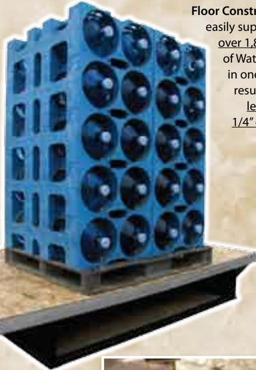
HEARTLAND's LAMINATED Floor Construction easily supported over 1,800 lbs. of Water Jugs in one spot - resulting in less than 1/4" of flex!!
