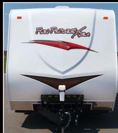
Front fiberglass cap with graphics, removable front storage tray and diamond plate rockguard.
