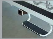
9 TOWING POSITION Step shifts to right – allowing for tow hitch and easy entry
