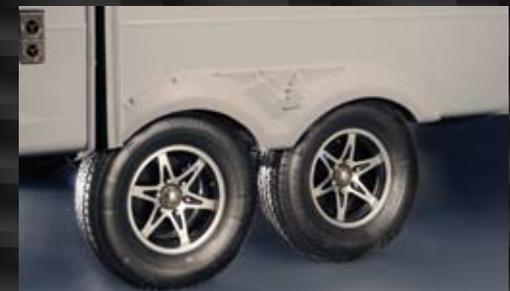
High Performance Aluminum Wheel Option. (15" with load range D, or 16" with load range E.)
