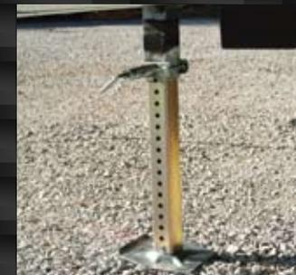
Hydraulic landing gear on Fifth Wheels (Optional) 10 times faster than conventional electric jacks. Quick release pins on Fifth Wheel feet. (Standard)
