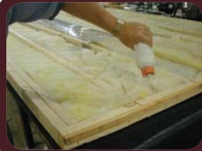
Gulf Stream constructs each coach using only the finest quality materials. The 5/8" floor decking is both glued and screwed to the sturdy 2x3 floor joists which are 13" on center and fully insulated. Then the floor assembly is bolted to the steel frame, providing one of the strongest floor systems on the market!
