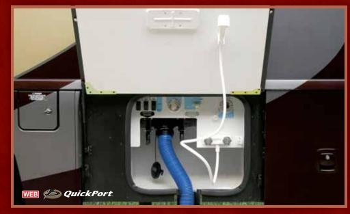
**SERVICE CENTER** Color-coded labels identify connection points and the QuickPort® service connection hatch makes connections fast and easy and allows the compartment door to be shut while connected to exterior service. The exterior shower is great for quick clean ups of muddy shoes or gear.
