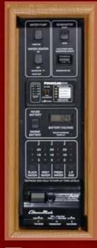
WEB ONE PLACE<sup>®</sup> Frequently used switches, gauges and controls can all be found in the OnePlace<sup>®</sup> systems center.
