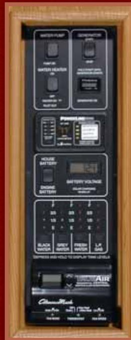
**WEB ONE PLACE®** Frequently used switches, gauges and controls can all be found in the OnePlace® systems center.
