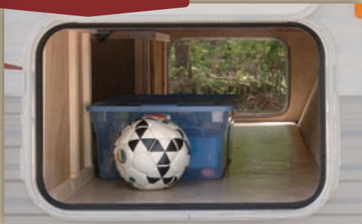
The pass-through design of the large, lockable storage compartments allows easy access to items from either side.
