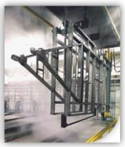
Corrosion-resistant frames are finished with a 12-stage E-Coat™ finishing system (select models)
