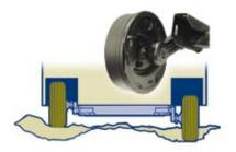
TorFlex® independent torsion-axle suspension gives more ground clearance, provides a smooth ride, makes towing easier and reduces wear and tear by absorbing bumps.
