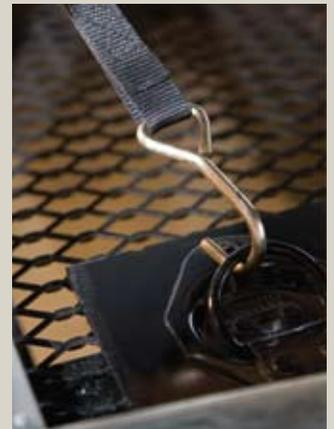
Six D-rings on the front deck safely secure your bikes or ATV.
