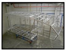
Host campers are 100 % aluminum framed, on 16 " centers, with all window, door and hatch openings individually framed for added strength and integrity.
