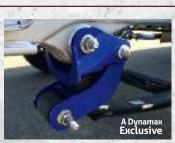
DynaRide provides a smoother ride than conventional leaf springs, and increases the ride height to be more effective. Rubber absorbs shock and protects from road damage.
