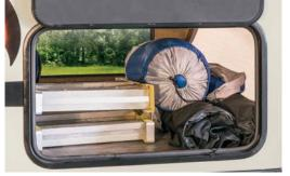
Oversized radius-cornered baggage doors with convenient magnetic catches.
