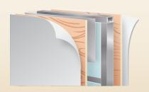
Using TuffShell™ vacuum-bonded lamination, our walls combine welded aluminum framing, fiberglass sidewalls and metal backers, ensuring your camper can handle the toughest conditions.
