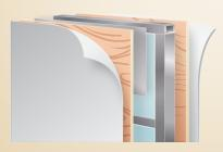
Using TuffShell™ vacuum-bonded lamination, our walls combine welded aluminum framing, fiberglass sidewalls and metal backers, ensuring your camper can handle the toughest conditions.
