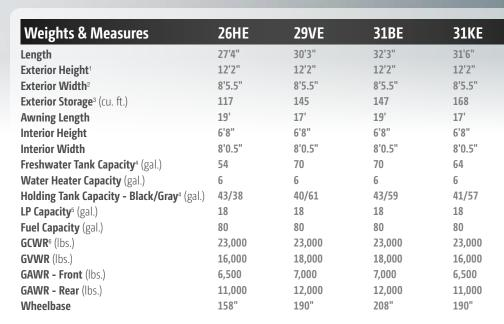
1 The height of each model is measured to the top of the tallest standard feature and is based on the curb weight of a typically equipped unit. The actual height of your vehicle may vary by several inches depending on chassis or equipment variations. Please contact your dealer for further information.
