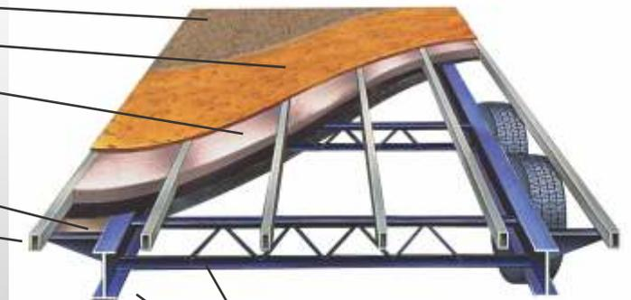
Heavy Duty Truss Chassis Supports I-Beam Chassis
