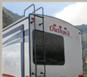
Rear roof ladder w/fully walkable roof
