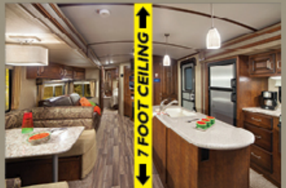
VAULTED CEILING 7' CENTER CEILING HEIGHT ALLOWS FOR ADDED HEADROOM, LARGER WINDOWS AND ADDED STORAGE
