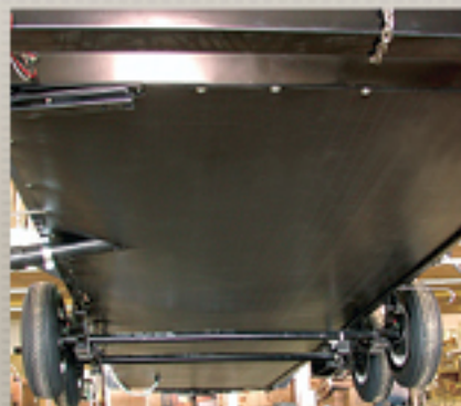
The Heated and Enclosed Underbelly extends the camping season and provides better tow ability.
