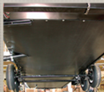
The Heated and Enclosed Underbelly
