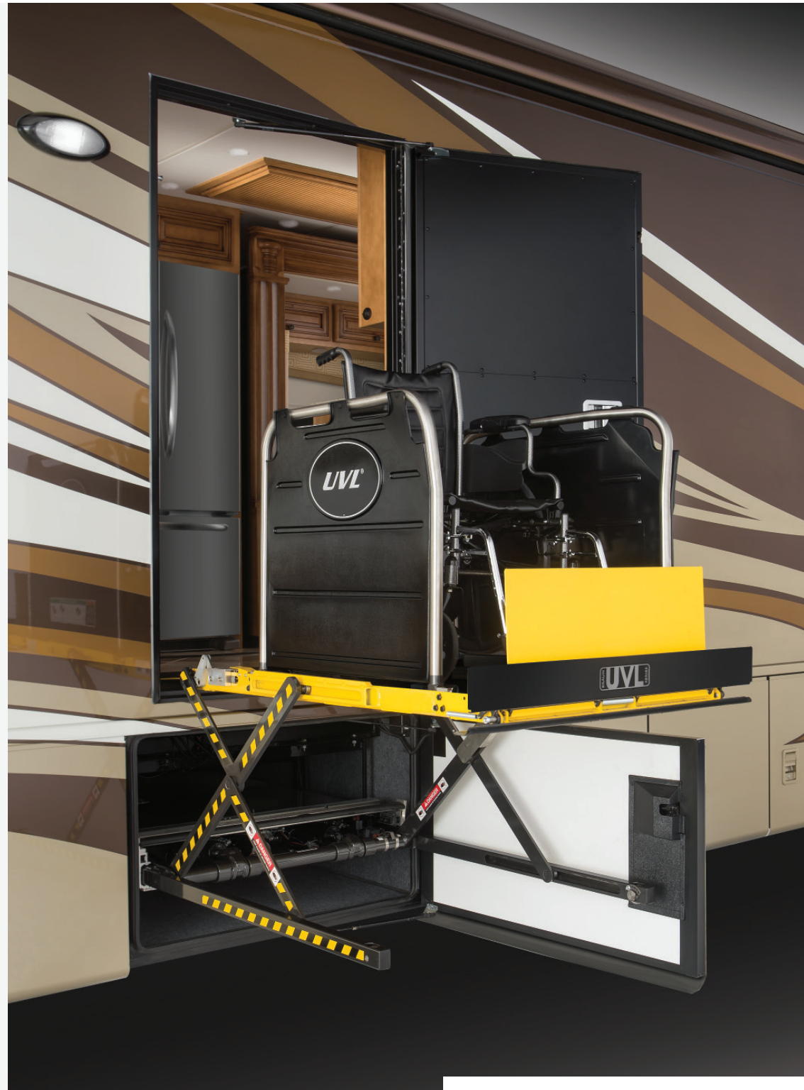
Remote-Control Lift with Access Door
