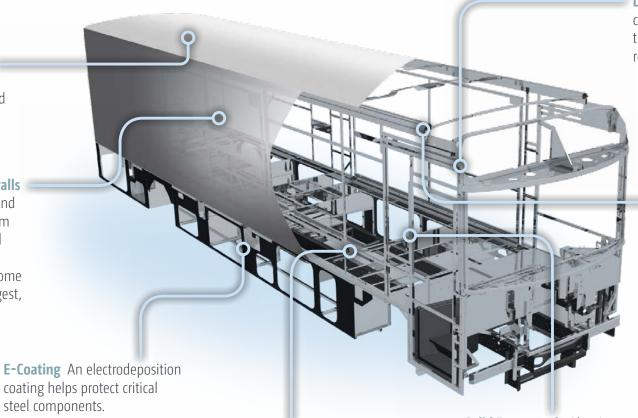
**Laser-Cut Tubing** Precision laser cutters create precise joints in structural steel that are stronger and require less welding.
