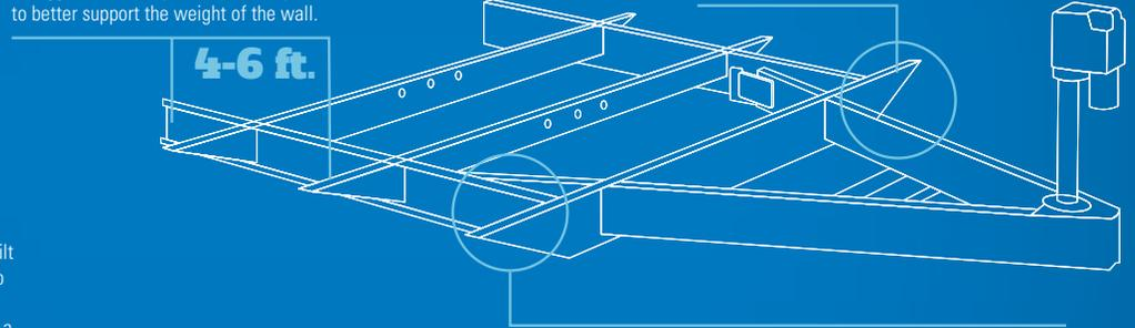
**Fifth wheel frame:** The frame over the truck bed is built on a superior 2-inch x 6-inch tube perimeter structure to better support the bedroom sidewalls. Competing fifth wheels have a smaller frame; these manufacturers add a sidewall support seam to compensate for expansion joints.
