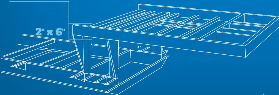
**I-class cambered structural steel I-beams:** Jayco uses a unique molded, one-piece design to prevent the unit from twisting; competing three-piece I-beams can warp over time at the welded seams.
